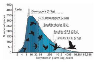
Figure 1. The frequency distribution of bird body masses (in grams) in relation to possible tracking technologies. Minimum bird sizes for each technology are represented according to the 5%-body-weight rule.
